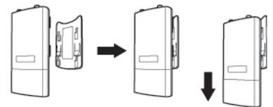
Installing Rocket M on RocketDish requires no special tools, you simply snap it securely into place with the universal Rocket mount built into the antennas.
